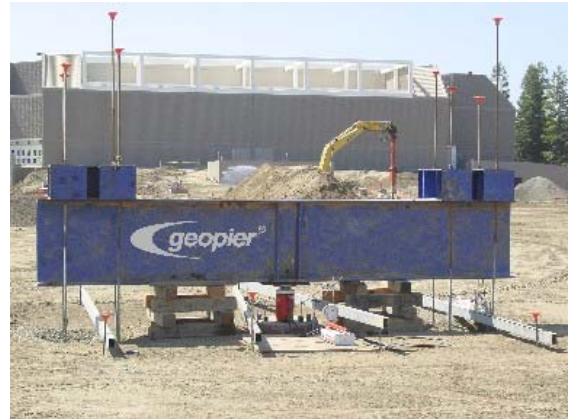
Fig. 7 Photo of RAP Modulus Test Set-up
