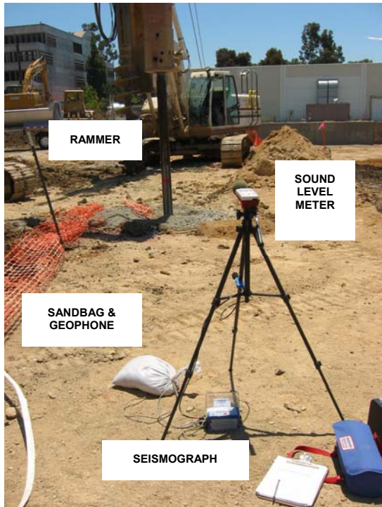
Fig. 4 Photograph showing typical instrumentation set-up.
